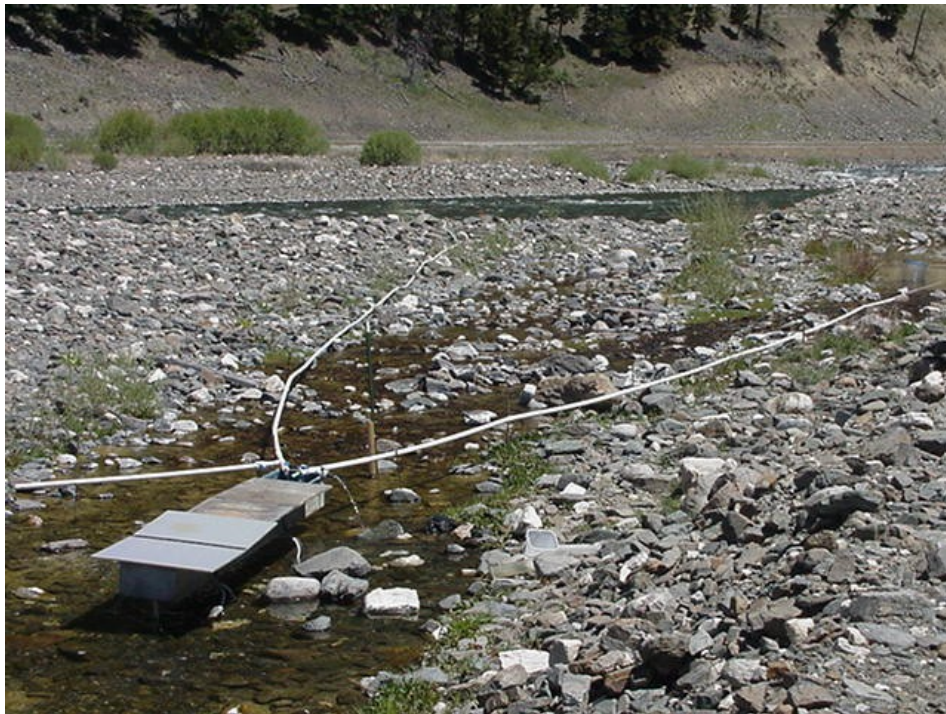
Figure 6. Trough system used to expose sentinel rainbow trout to various concentrations of Whirling Disease TAMS at the South Slide side channel in 2001.
