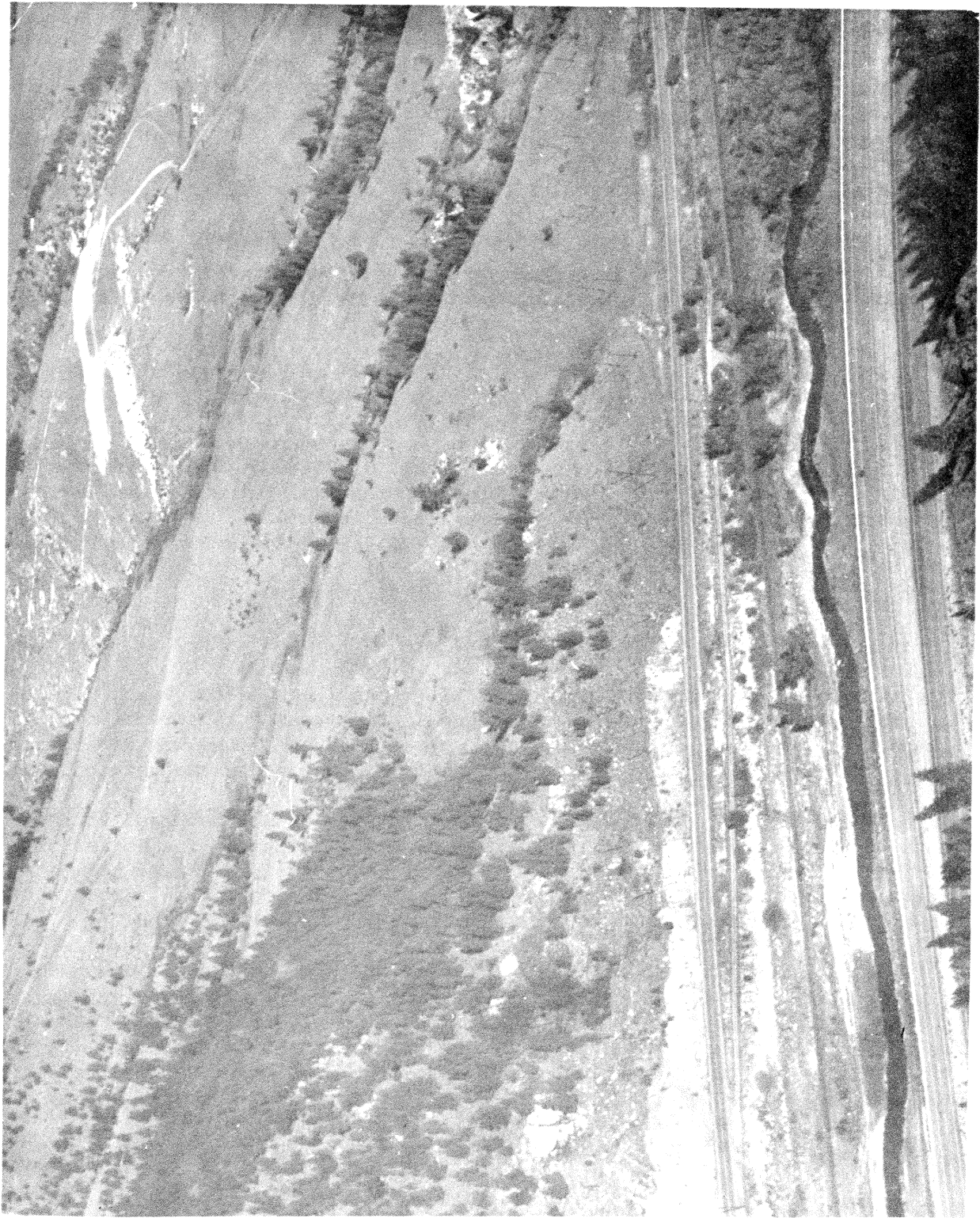
FIGURE 1. Photograph of artificial channel on Prickly Pear Creek showing man-made meanders.
