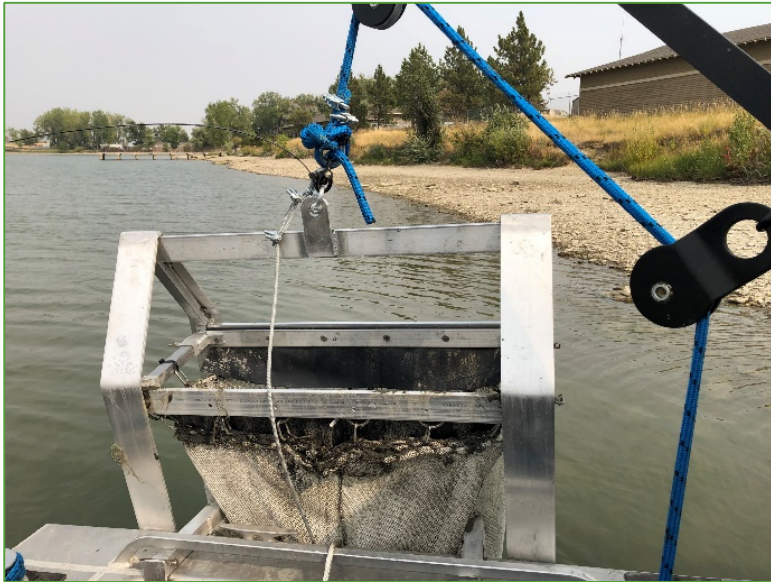
Figure 20. Benthic sled that is dragged behind the boat to sample for Asian clam at Lake Elmo. It will let sediment through while trapping anything larger than 1/8".
