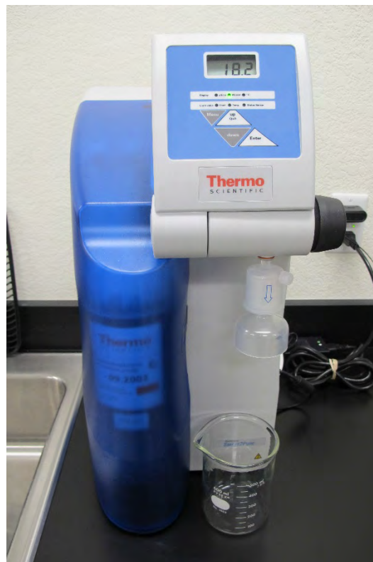
Figure 19: Deionizing water filtration system
